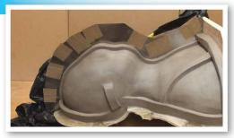
I cut it into 2" strips and push them into the clay down the middle to quickly create a dividing wall. I used parcel tape to strengthen it, and placed it in the middle of the central key where the clay is thickest.
