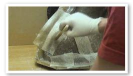
Then I put the first layer of glass over the keys and the edges first.
