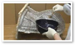
Then it's time for the laminating resin. It gets worked into the chopped strand and creates a nice layer to put the strips of wetted out glass onto.
