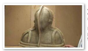
After this, I wash the mould down with water to get rid of any dust on the surface and the fibreglassing for this mould is finally finished.
