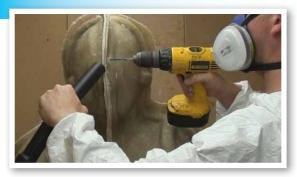
Before I open this up, I need to drill the holes for the bolts I will use later to hold this mould together.
