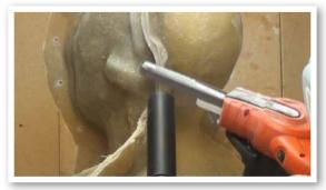
It generates a lot of dust so I use extraction as well as this workshop vacuum to keep the dust levels down.
