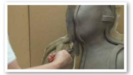
Once the edge is trimmed, I need to carefully pull out the shim wall. It is possible that you could just leave it and glass the other side, but I prefer to remove it.
