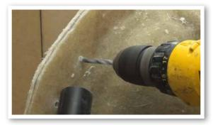
It's important to use extraction and appropriate protective gear to prevent the fibreglass dust being inhaled.
