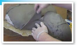
Make sure the clay covers everywhere, and cut or bend the clay to fit any gaps.
