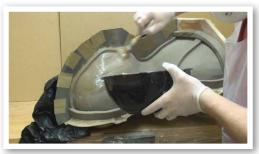
The gelcoat is mixed and applied just as before in the first video, with a little extra catalyst to compensate for the cool and damp clay.
