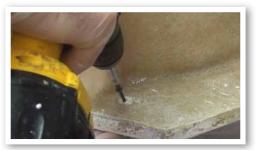
I want to make sure that the mould stays secure, so I drill three small pilot holes through the glass and into the base so I can screw this in place.
