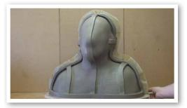
Once the edge has a key all the way around, I placed a few bigger keys on the head to help the silicone locate better there.
