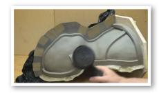
I release this shim wall and the clay using a spray wax and dry it using a blow dryer ready for gel coating.
