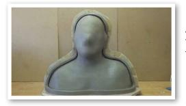
Any gaps should be filled so you create a neat low wall like this all around the edge. This will act as a key to locate the silicone in it's jacket later.
