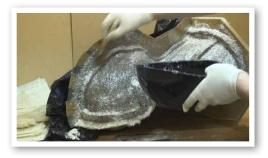
The resin I use for laminating is mixed next, and the first job is to wet the chopped strands, and make sure there is no dry glass left.
