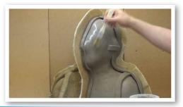
I need to release the exposed fibreglass and clay so the gelcoat will release easily, and I use a liquid wax and dry this with a blow dryer. As an extra precaution, I also give it a coat of spray wax just to be sure.
