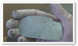
Using a serrated kidney like this, I can even out the surface by lightly dragging it over the clay and take out any bumps.
