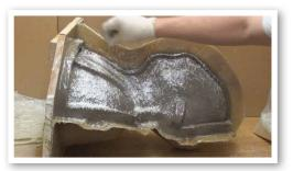
Once the gelcoat has set up enough, the chopped strands go on. It may be necessary to tilt the head upright again to get an even covering over the gelcoat.
