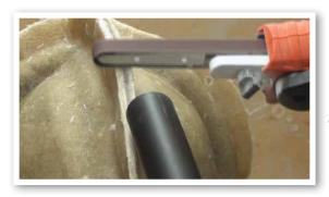
I also want to neaten these edges which are a little bit rough from the green trimming still. I am using a powerfile, a small belt sander which is ideal for this job.
