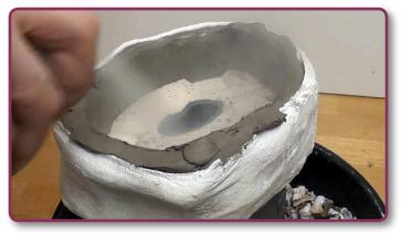
Dropping a little plaster into the deepest part first, tap and roll the mould to push out any air you might trap, and gradually top it up until there is a nice solid block.
