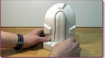
Drilling three holes around the base with a 6mm drill bit will allow me to inject the silicone in here and allow the air the silicone will displace to escape
