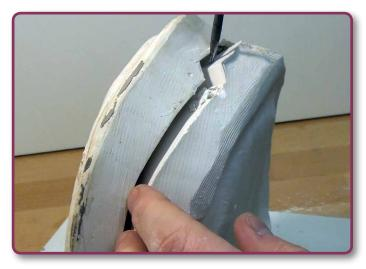
So now we have our two mould halves. There is a little damage from the screwdriver, but this isn't a problem. The mould is made thick enough to take this.
