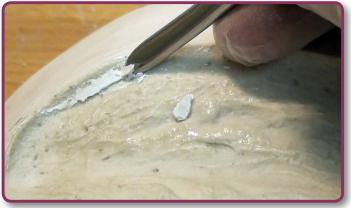
By popping half the mould on, you can see how the tongue core sits perfectly, floating in the middle and leaving a gap all the way around.
