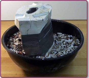
A quick clay wall is added and supported with bandage like before. This will enable the core to sit
