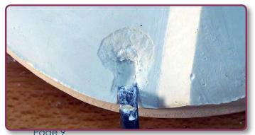
Shaving down any sharp edges is easily done with a rasp tool called a surform. Rifflers such as these are also good for awkward areas.
