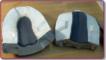
Once both halves are done, check that the mould can still close up correctly, and then secure the two halves together with a strong duct tape or bungee cord. These methods are more convenient than clamps.
