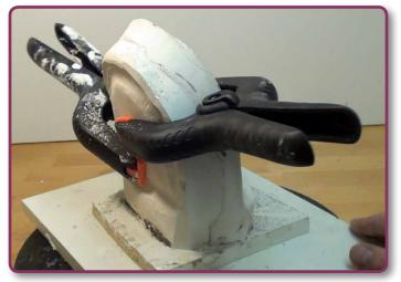
The next morning, I open the mould up. You can clearly see the seam line between the two halves. By driving a screwdriver into this seam carefully. I can pop the two halves apart.
