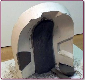
Once again, I add a wall around the edge and spray more wax release. Allow it to dry thoroughly, and it will stop the new plaster section I am about to add from bonding to this one.
