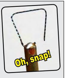
**One note:** this repair depends on the loop breaking at the base where it joins the handle - if the loop breaks in the middle then I think replacing the actual loop itself is the best option, or making a new tool from scratch. If so inclined then check out my tutorials on making loops and wooden tools.
